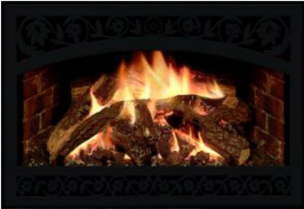
*Burner Flame Heights:* This image provides a visual reference for the burner flames burning at maximum height after the burners have been operating for 30 minutes or longer. A normal rear flame will be 1 to 2 inches above the rear log top edge. This, however, is dependent on the gas type, air shutter opening setting and vent system configuration. Actual flame heights can be slightly higher or lower when compared to this reference image.
